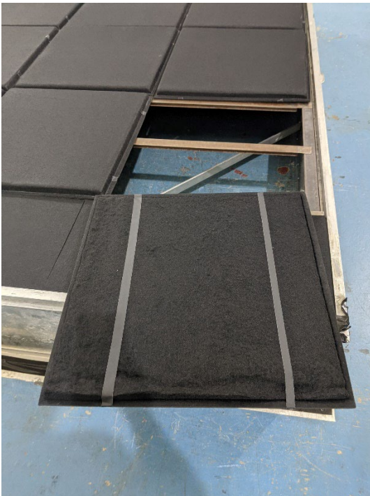
Figure 2 – Detail of 1” fill attached to specimen drop panel with straps
